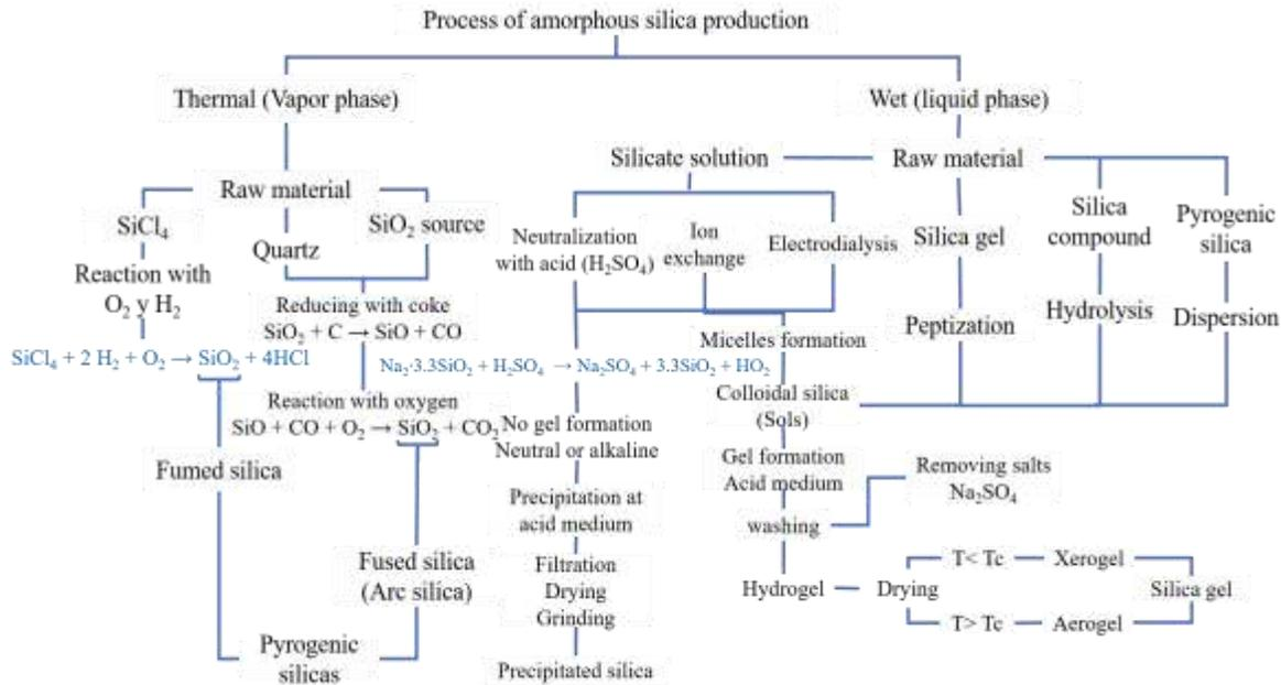
**Figure 1.** Different commercial silica routes of production (adapted from [45]).
