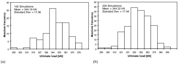
Figura 5. Histogram for the ultimate load.  $L_e = 3m$ . (a) 100 simulations, (b) 200 simulations.
