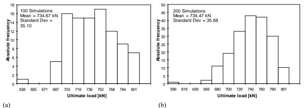
**Figure 3.** Histogram for the ultimate load.  $L_e = 2m$ . (a) 100 simulations, (b) 200 simulations.
