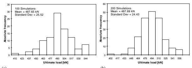
(a) (b) Figure 4. Histogram for the ultimate load.  $L_e = 2.5$ m. (a) 100 simulations, (b) 200 simulations.
