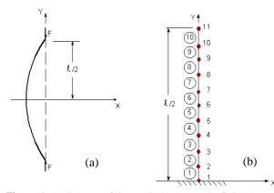
**Figure 1.** (a) Scheme of the studied column, (b) finite element model.
