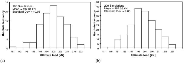
Figura 6. Histogram for the ultimate load.  $L_e = 4m$ . (a) 100 simulations, (b) 200 simulations.
