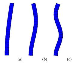
Figure 2. (a) Mode 1,  $P_{CRI} = 791$ kN, (b) Mode 2,  $P_{CR2} = 7117$ kN, (c) Mode 3,  $P_{CR3} = 19794$ kN
