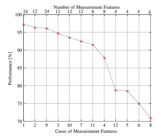
Figure 4. Cases and number of measurement features vs performance values for single phase to ground fault, phase a. Source. Own elaboration.
