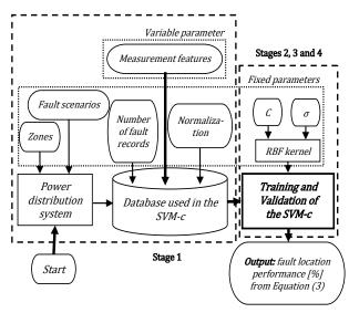
Figure 2. Block diagram of the implementation of fault locator method for non-linear cases. Source. Own elaboration.
