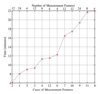
Figure 5. Cases and number of measurement features vs time values for single phase to ground fault, phase a.
