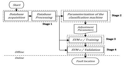
Figure 1. General scheme of the classification method. Source. [13].
