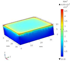
Figure 4. Applied load according to the geometries of piezoelectric material - flat plate.
