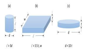
Figure 1. Design features of different geometries of piezoelectric material. (a) Pole rod, and (b) thin flat plate and (c) thin flat disc.
