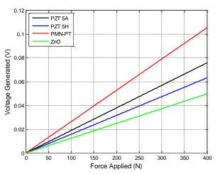
Figure 7. Voltage generated by applied load according to the geometries of piezoelectric material - thin flat plate.
