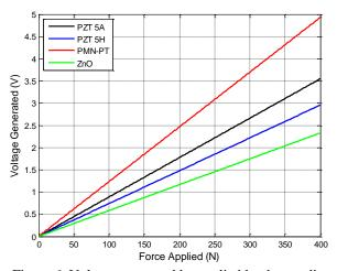
Figure 6. Voltage generated by applied load according to the geometries of piezoelectric material - Pole rod.
