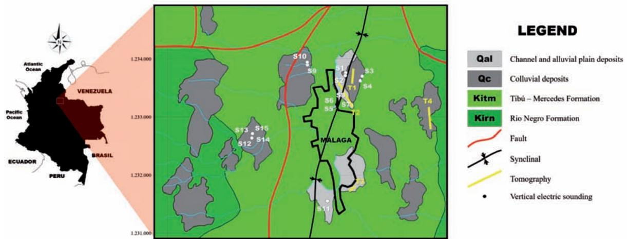
FIGURE 1. Localization of study area, showing the distribution of electrical resistivity tomography (T) and vertical electrical sounding (S) sites.
