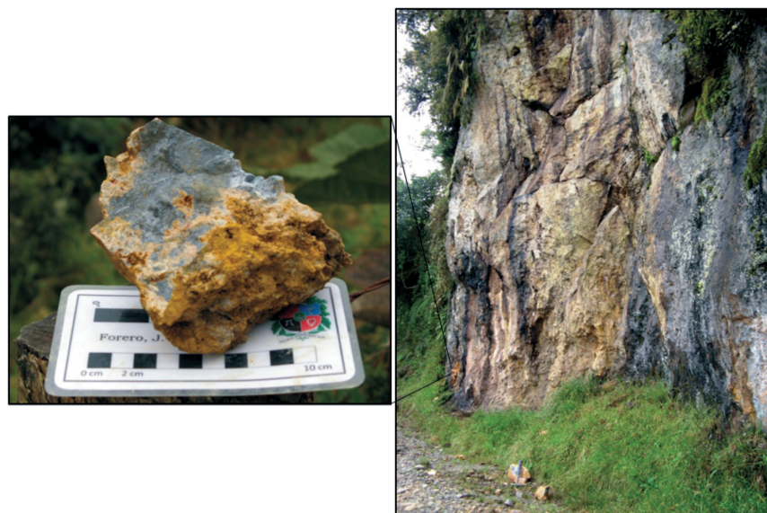
FIGURE 7. Silicification controlled by Villamaria-Termas fault system in locality GNR-JF-028, note the subvertically aligned oxidation pattern (right). In the left picture a hand sample (GNR-JF-028A) of silicified rock with a leached oxidation cap.
