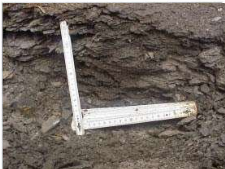
FIGURE 4. Laminated mudstone facies (LMS). Black to dark brown finely laminated organic-rich mudstone. Laminae are 1 - 2 cm thick weather as flakes or blocks. Folding ruler segment is 21.7 cm. Location: Breached Anticline section.
