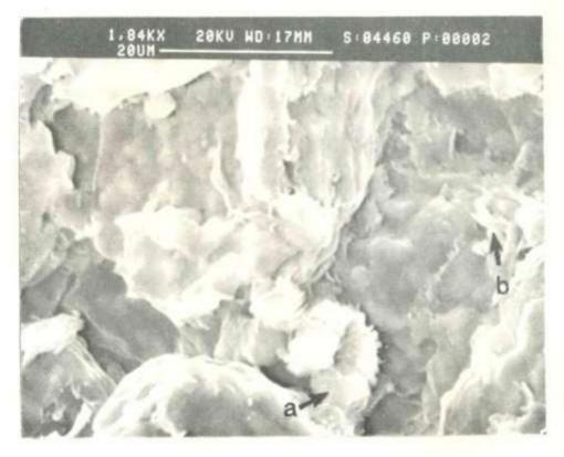
Plate 4-3 SEI photomicrograph of crystalline kaolinite booklets (a) plugging a pore throat. Note that the grain surfaces are otherwise free of clay.
