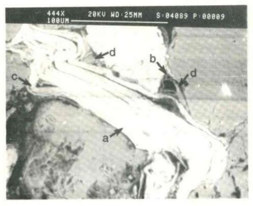
Plate 3-2 BEI photomicrograph showing a splayed mica (a). Note that the splaying of the mica has closed pore throats (b) and will reduce interconnectivity between macropores. K-feldspar grains have undergone partial dissolution and grain collapse (c).
