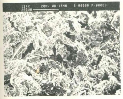
Plate 1-3 TS photomicrograph of a coarse silt to very fine sand grade, moderately well sorted (visually estimated) subfeldspathic wacke. The siltstone is essentially non-porous but has discontinuous coarser grained laminae (a) with primary macropore systems.
