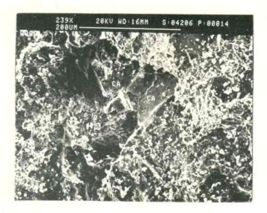
Plate 5-4 SEI photomicrograph of calcite (Ca) partially filling a pore and blocking pore throats. Note that the framework quartz grains (Q) do not have overgrowths and pores are generally clean.
