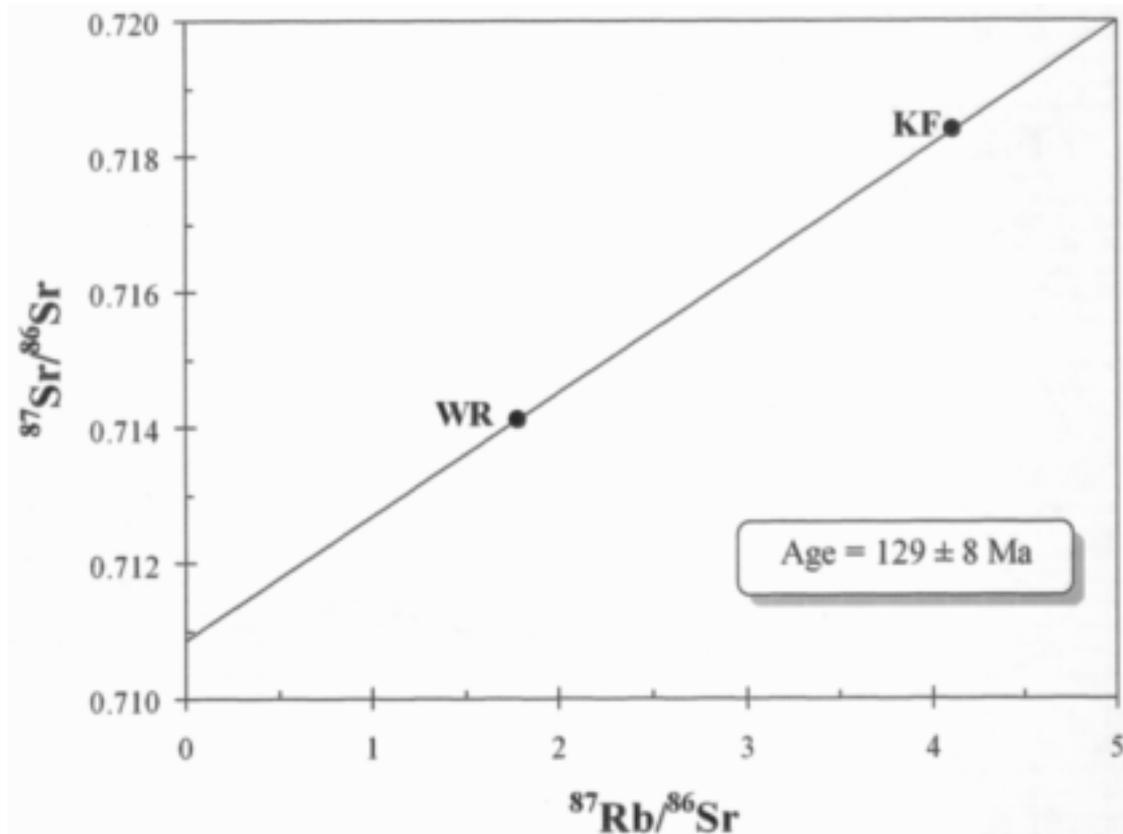
FIGURE 5. Rb-Sr whole-rock mineral isochron. WR = whole rock; KF = K-feldspar.
