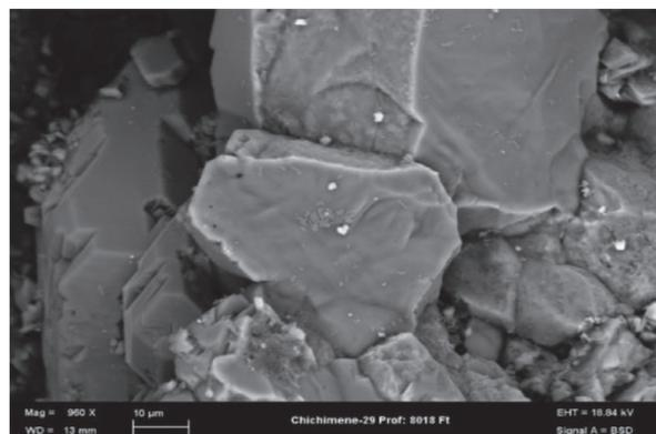
**Figure 9a.** SEM picture of plug inlet face.
