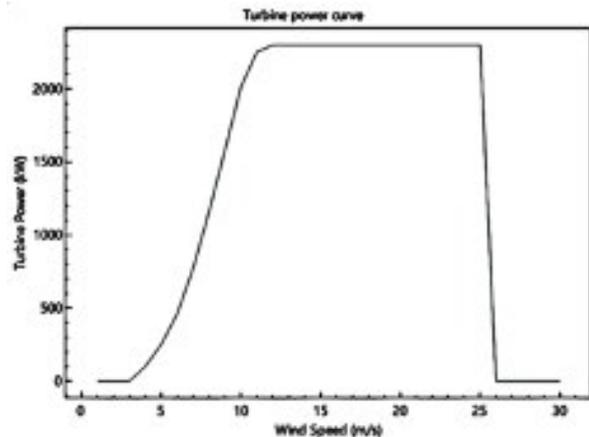
**Figure 3.** Turbine power as a function of wind speed
