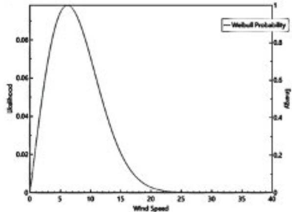
**Figure 2.** Likelihood and energy load curve as a function of wind speed. Source. The authors.
