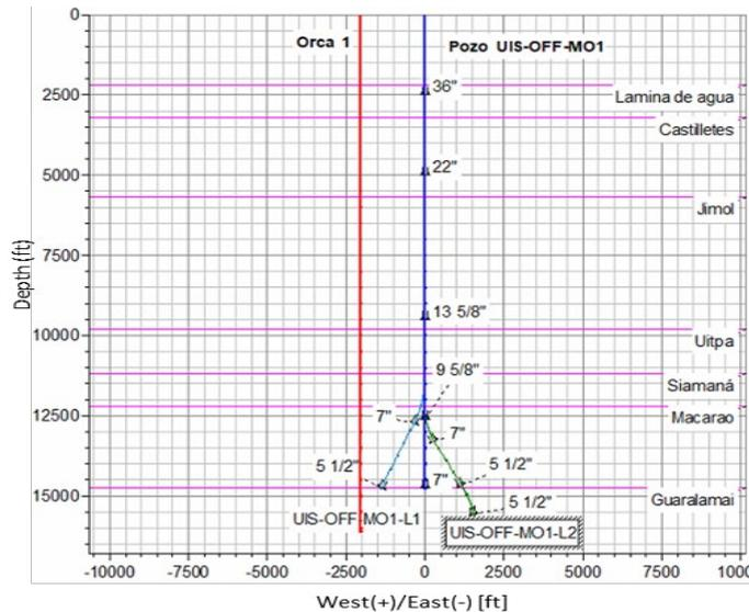
**Figure 14.** Front view of Orca-1 well and the UIS-OFF-MO1 multilateral well.
