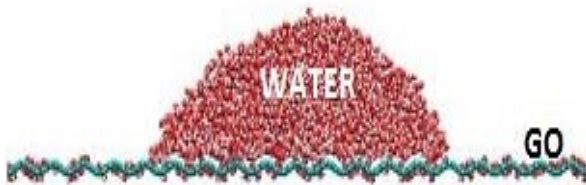
Figure 9. Diffusion of a water drop through corrugated layers from graphene oxide. (Nurrohman et al., 2023).
