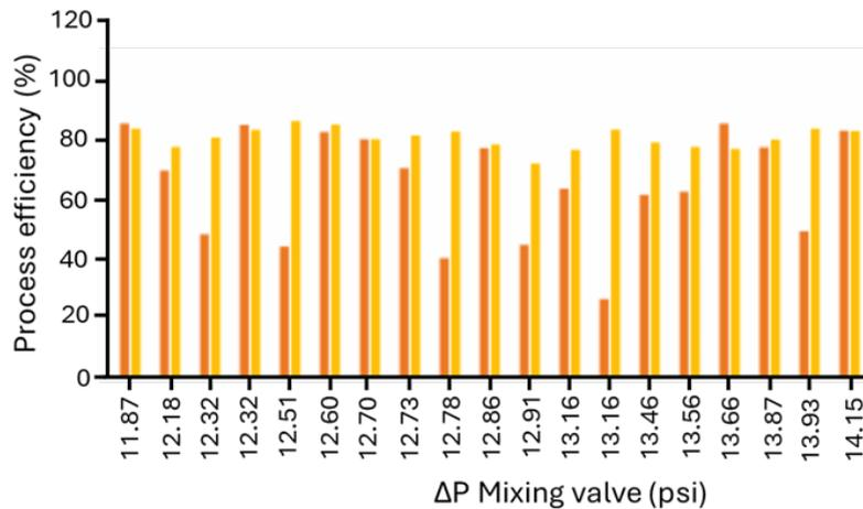
Figure 6. Dehydration and desalting efficiency in D-001.
