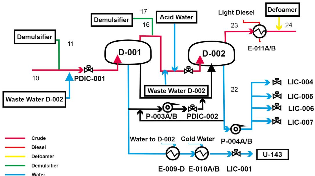
**Figure 3.** Two-stage desalting and dehydration unit.
