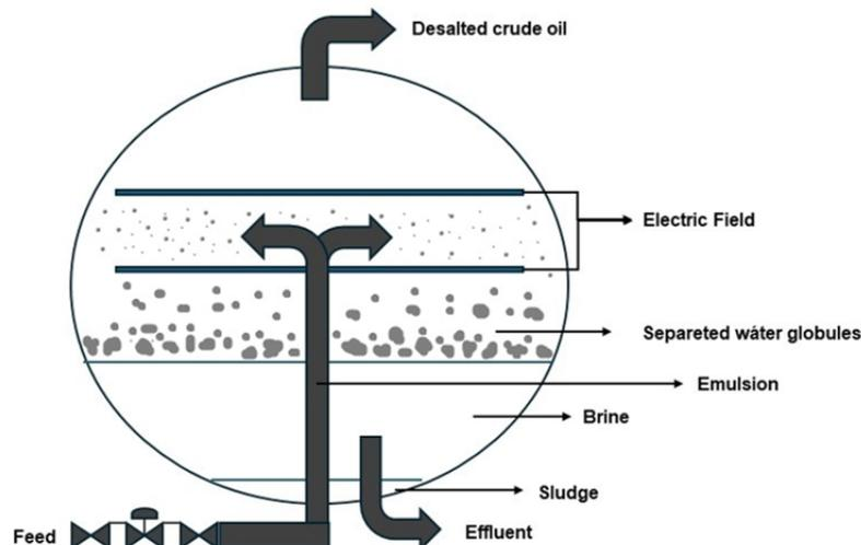
Figure 2. Operation of electrostatic desalination.
