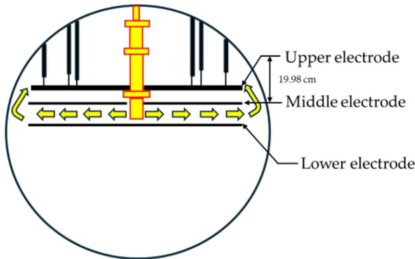
Figure 4. Desalinador cross section.
