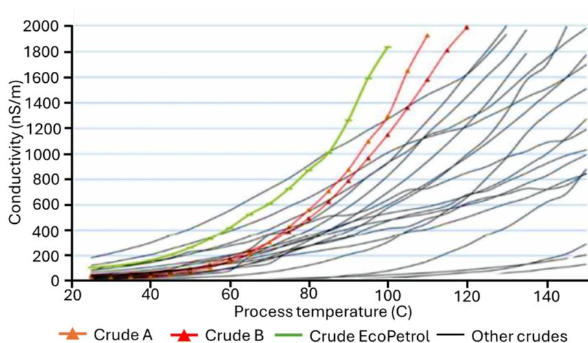
Figure 8. Conductivity of crude oil in refinery.
