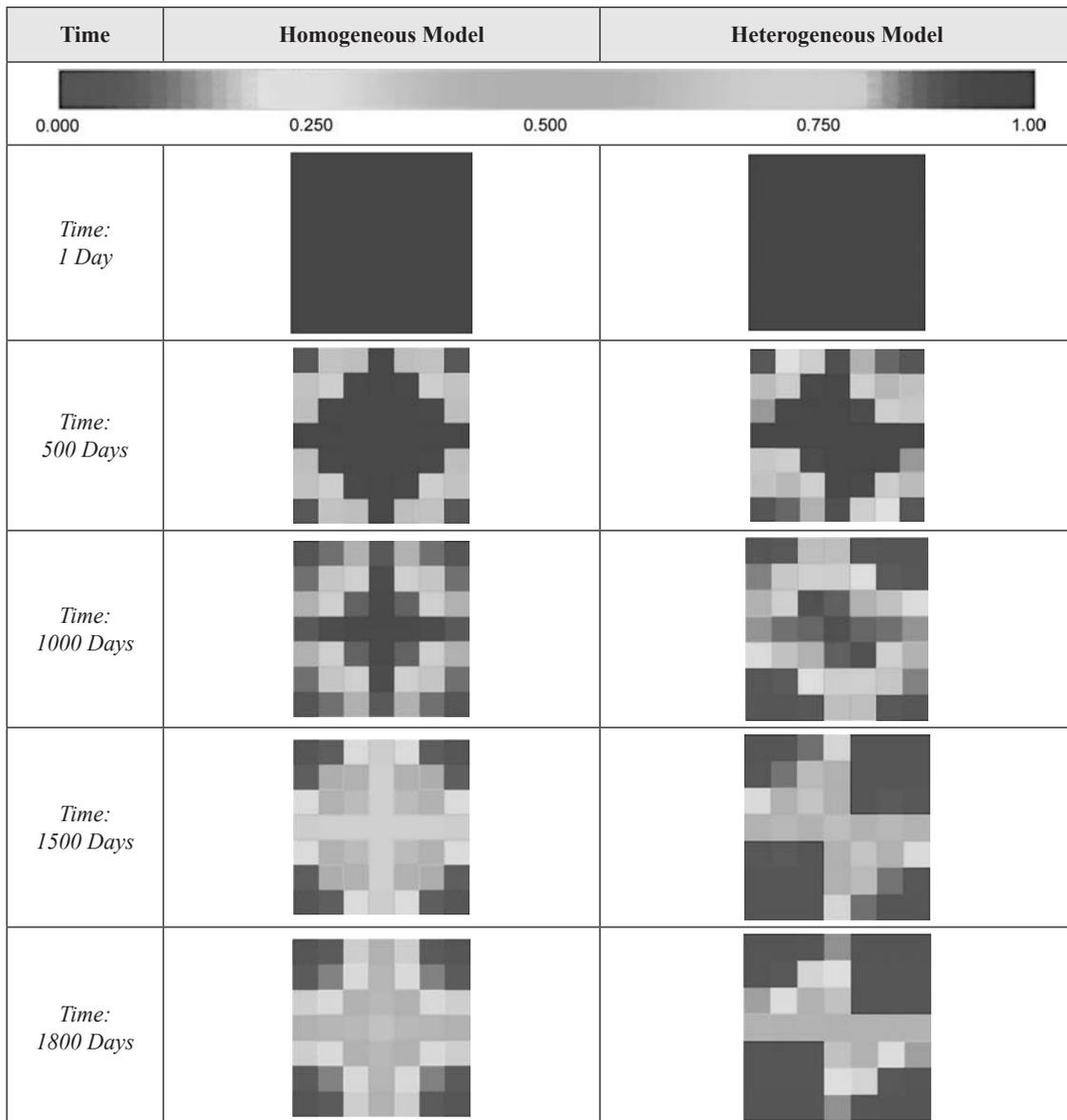
Fig 5. Oil saturation in the fracture system
