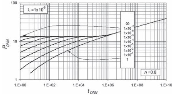
**Figure 2.** Effect of the dimensionless storage coefficient on the pressure response of a heterogeneous reservoir
