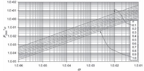
**Figure 8.** Values of the dimensionless pressure times the dimensionless storage coefficient against storage coefficient for several values of the flow behavior index
