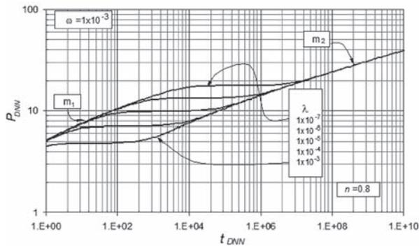
**Figure 3.** Effect of the interporosity flow parameter on the pressure response in a heterogeneous reservoir
