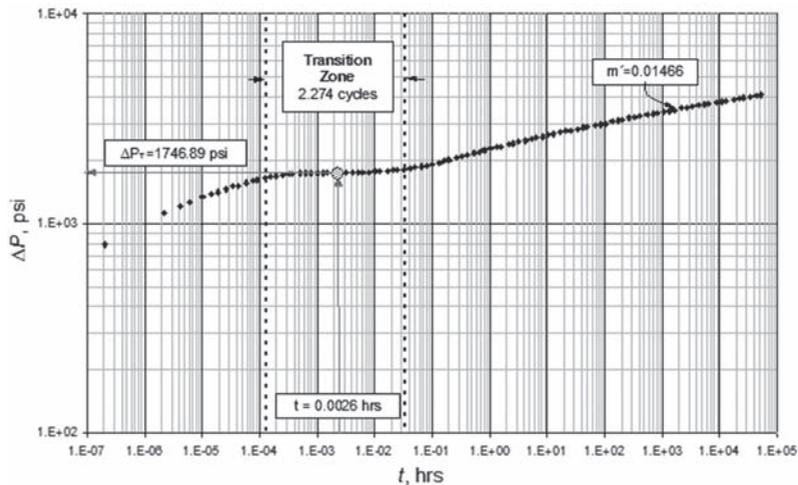
**Figure 11.** Log-log plot of  $\Delta P$  vs.  $t$  for example 3
