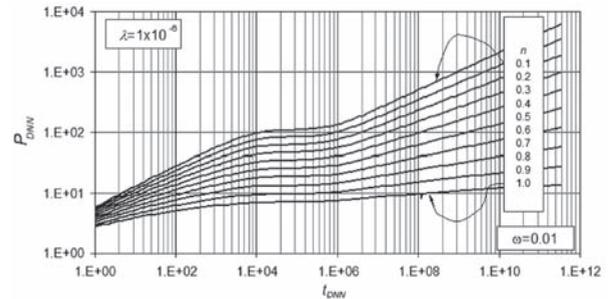
**Figure 4.** Effect of flow behavior index on pressure response in a heterogeneous reservoir
