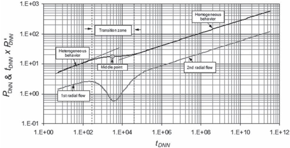
**Figure 1.** Dimensionless pressure and pressure derivative log-log plot displaying the typical behavior of a dual-porosity reservoir for  $\omega=0.01$ ,  $\lambda=1 \times 10^{-7}$  and  $n=0.25$
