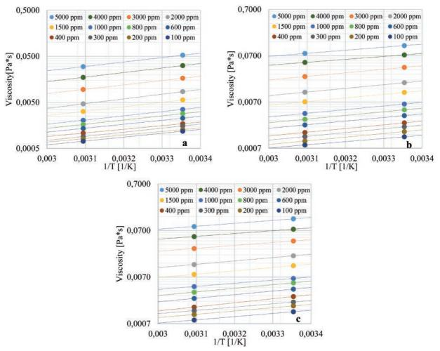
**Figure 5a-c.** Arrhenius plot of viscosity at a different concentration with shear constant  $\gamma = 7.8s^{-1}$ , **a** HPAM Solution with SB I; **b** HPAM with SB II; **c** HPAM with SB III.
