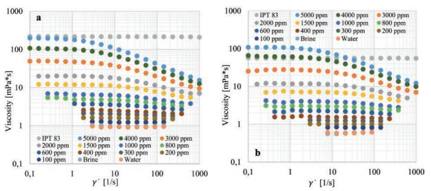
Figure 3a, b. Viscosity vs. Shear Rate for Polymer Solution with Synthetic Brine II and different polymer concentrations at a 298.15 K; b 323.15 K.
