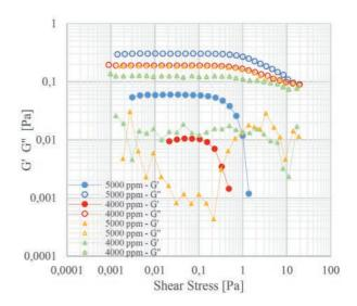
Figure 9. AST results. G' G'' vs. Shear Stress of HPAM solution with SB I. Where the Circle corresponds a temperature of 298.15 K, and the triangle corresponds a temperature of 323.15 K.
