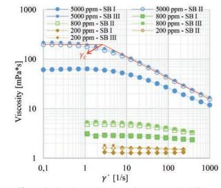
Figure 6. Viscosity vs. Shear Rate for HPAM with different SB composition and three different polymer concentrations (SB I: Na<sup>+</sup>, Cl<sup>-</sup>, K<sup>+</sup>, Ca<sup>+2</sup>, Mg<sup>+2</sup>; SB II: only Na<sup>+</sup>, Cl<sup>-</sup>; SB III: Na<sup>+</sup>, Cl<sup>-</sup> and HCO3<sup>-</sup>), at 298.15 K.
