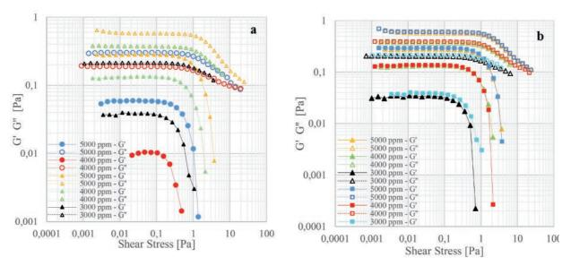
Figure 8a, b. AST results. G' G'' vs. Shear stress at 298.15 K. Where the Circle represents HPAM solutions with SB I, the triangle represent HPAM solutions with SB II and the square represents HPAM solutions with SB III.
