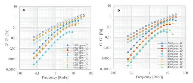
Figure 11. a, b. FST results. G' G'' vs. Shear Stress of HPAM solution with SB II and SB III, respectively. The Circles correspond to 298.15 K, while the triangles correspond to a temperature of 323.15 K.
