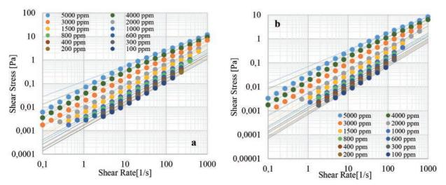
Figure 1a, b. Shear Stress vs. Shear Rate for HPAM Solution with Synthetic Brine I and different polymer concentrations at a 298.15 K; b 323.15 K. Dashed lines - Carreau-Yasuda fits, continuous lines - Ostwald-de Waele fits.
