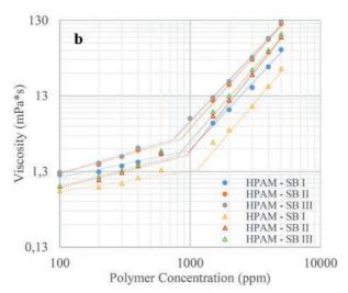
**Figure 7b** Viscosity vs. Polymer concentration for different Brine compositions at  $\gamma = 7.8s^{-1}$ . Where the **Circles** are T=298.15 K and **triangles** are T=323.15 K.
