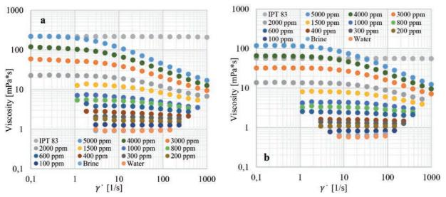
Figure 4a, b. Viscosity vs. Shear Rate for Polymer Solution with Synthetic Brine III and different polymer concentrations at a 298.15 K; b 323.15 K.
