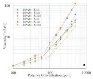
**Figure 7a.** Viscosity vs. Polymer concentration for different Brine compositions at 298.15 K. Where the **Circles** are  $\gamma = 7.8s^{-1}$  and **triangles** are  $\gamma = 143s^{-1}$ .
