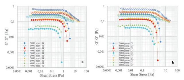
Figure 10. a, b. AST results. G' G'' vs. Shear Stress of HPAM solution with SB II and SB III, respectively. The Circles correspond to 298.15 K, while the triangles correspond to a temperature of 323.15 K
