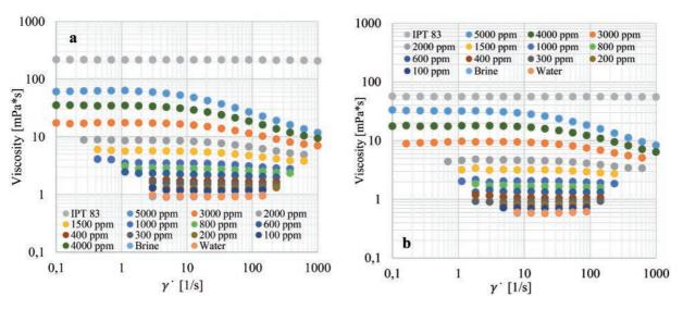
Figure 2a, b. Viscosity vs. Shear Rate for HPAM Solution with Synthetic Brine I and different polymer concentrations at a 298.15 K; b 323.15 K.
