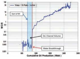
Figure 7. WOR versus Cumulative Oil Production.
