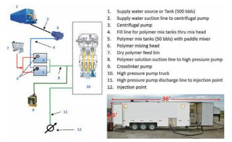
Figure 13. Field Application Schematic & Pumping Equipment.
