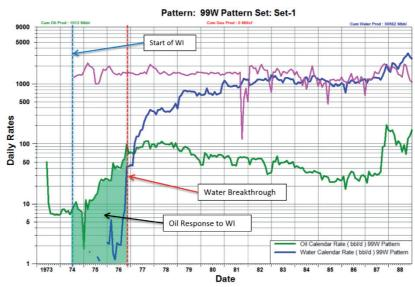
Figure 3. Basic production - injection data analysis.
