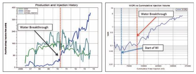
Figure 4. Injection drive-fluid breakthrough.
