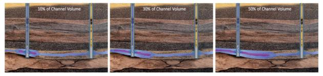
Figure 9. Importance of Bulk Gel Treatment Volume.
