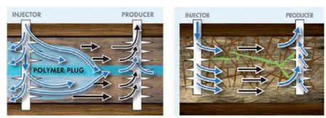
Figure 8. Redistribution of injected water after Bulk Gel.
