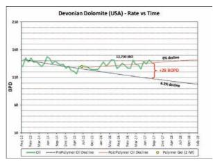
Figure 16. Oil rate vs Time
