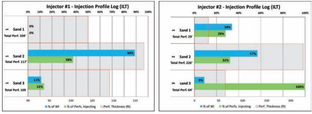
Figure 6. Injection profiles logs.
