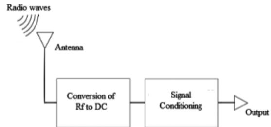
**Figure 1.** Based energy harvesting system RF [6].
