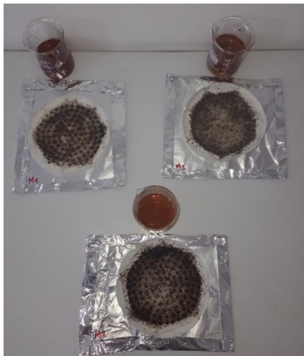
Figure 7. Dried acid-insoluble lignin together with the hydrolysate obtained.
