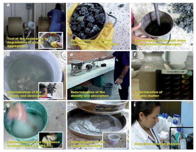
Figure 4. Procedures used for testing.
