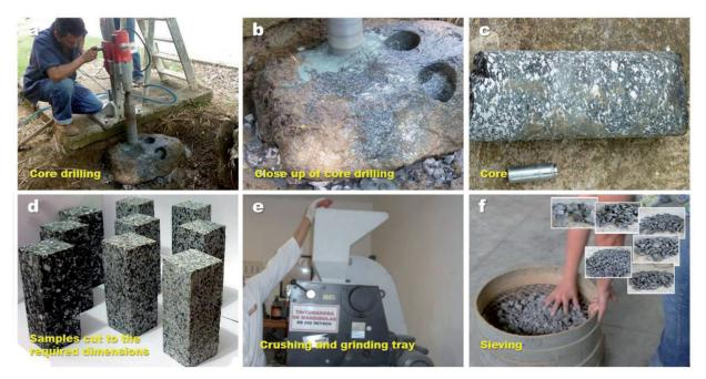
Figure 3. Stages during sample preparation.
