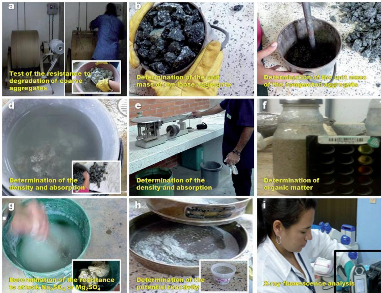
Figure 4. Procedures used for testing.
