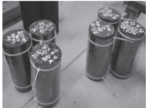
Figure 2. Protection around samples to ensure top face exposition.
