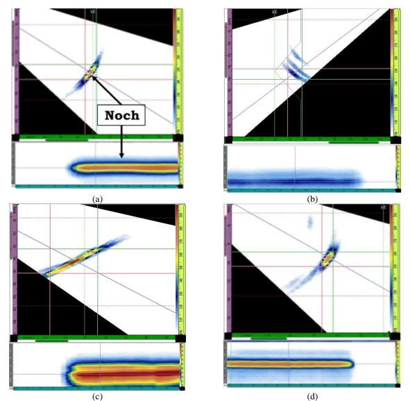
Figure 2. S-scan (top) and C-scan (bottom) displays. (a) M4, Skew 90°, Angular resolution: 0.5°, without focusing.
