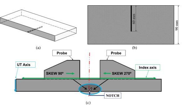
Figure 1. Schematic of the mechanized samples. (a) three-dimensional view. (b) Top view with dimensions in mm. (c) probe locations on inclined notches. Source: own elaboration.
