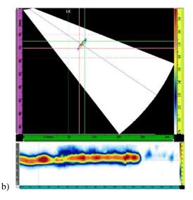
Figure 3. Inspection results at point 4 of sample welded with 0.5 ° angular resolution. (a) focused on 3 mm. (b) without focusing the ultrasonic beam. Source: Own elaboration.
