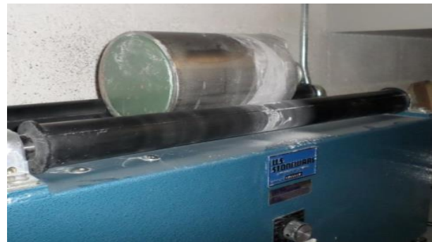
Figure 1. Wet grinding process in a laboratory ball mill. Source: Mill room SIU - UdeA
