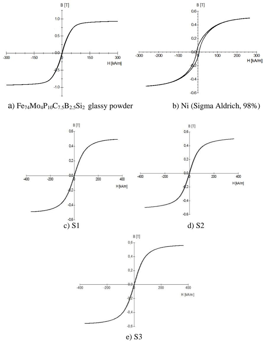
Figure 3. Hysteresis loops of the tested samples
