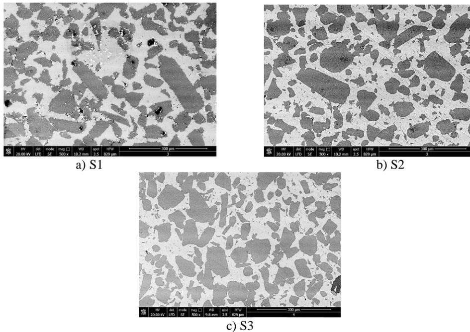
Figure 1. SEM morphologies of the hot-pressed samples
