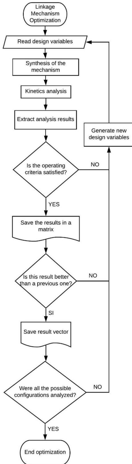
Figure 8. Optimization code flow diagram. Source: self-made.
