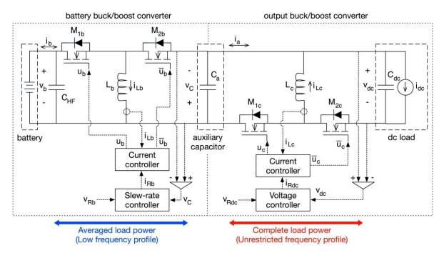
Figure 1. Double-stage battery power system
