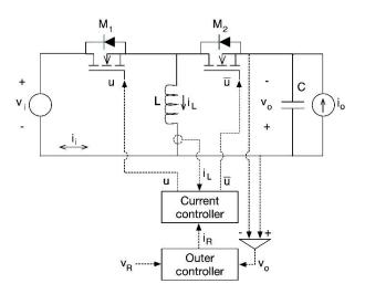
Figure 2. Circuital model of a single buck/boost stage.
