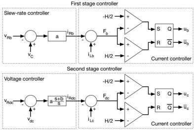
Figure 5. Implementation of the power circuit controllers
