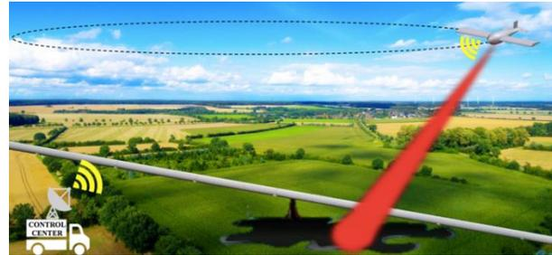
Figure 3. The schematic view of the UAV using a small infrared camera and a communication system.
