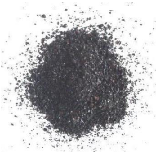
Figure 2. Blast furnace dust (BFD)
