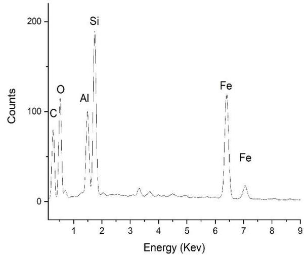
Figure 3. General EDS spectrum of the particles obtained magnetically from fly ash. Source: authors.
