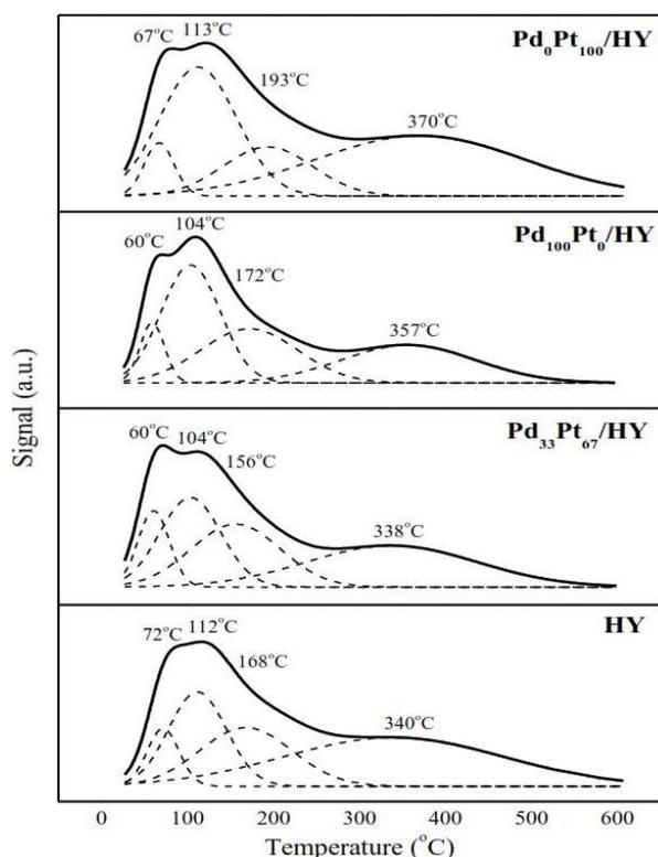
Figure 2. Thermodesorption of ammonia (NH<sub>3</sub>-TPD) on Pd-Pt/HY catalysts.
