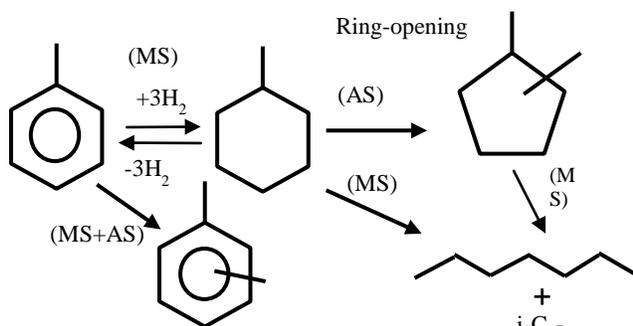
Figure 6 he hydrogenation of toluene to methylcyclohexane in metal sites and subsequent skeletal isomerization.
