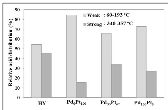
Figure 3. Relative Acid distribution (%) by NH<sub>3</sub>-TPD on Pd-Pt/HY catalysts.
