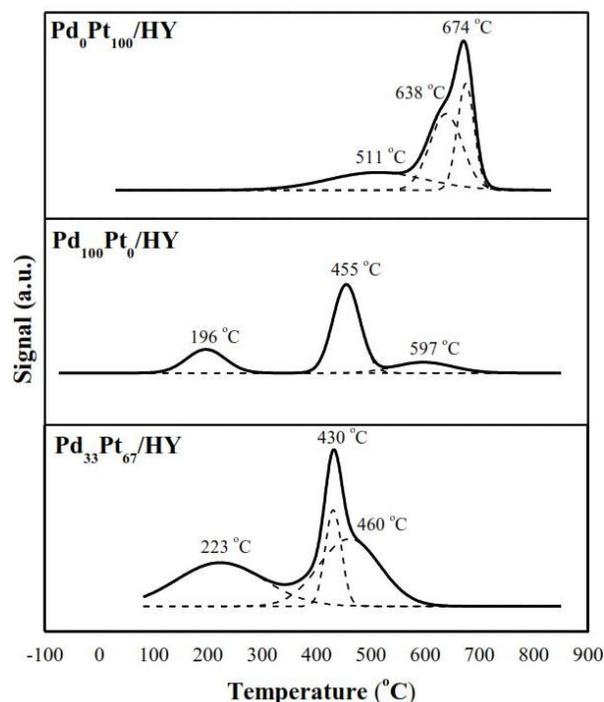
Figure 1. Hydrogen temperature-programmed reduction (H<sub>2</sub>-TPR) on Pd-Pt/HY catalysts.
