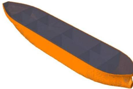
Figure 5. 3D hull model incorporating the wet surface of the FPSO vessel, which is elaborated through Sesam GeniE software.
