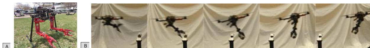
Figure 8. Development of manipulators adjusted to the UAV chassis, and their interaction with objects in space.
