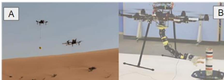
Figure 7. UAM grasping a moving object. Source: A) Vrba et al. [57], B) Zhang et al. [61].
