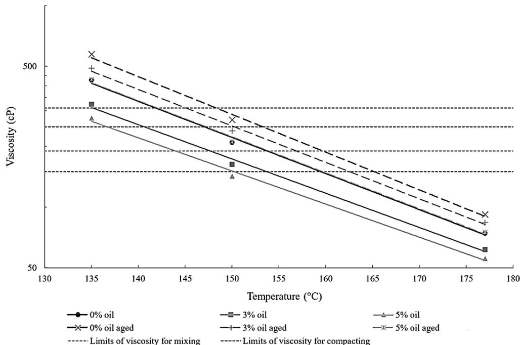
Figure 1. Trend lines of viscosity versus temperature.
