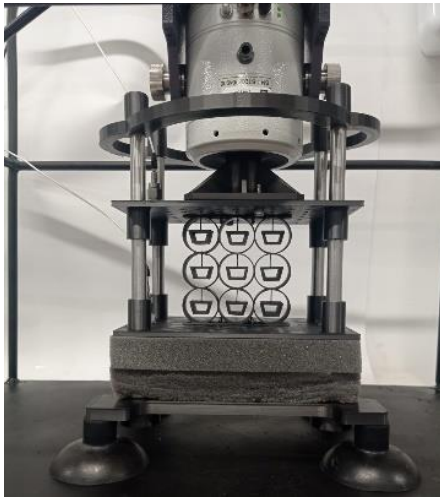
Figure 14. Assembly of the test bench to obtain the coefficient of transmissibility. Source: self-made.
