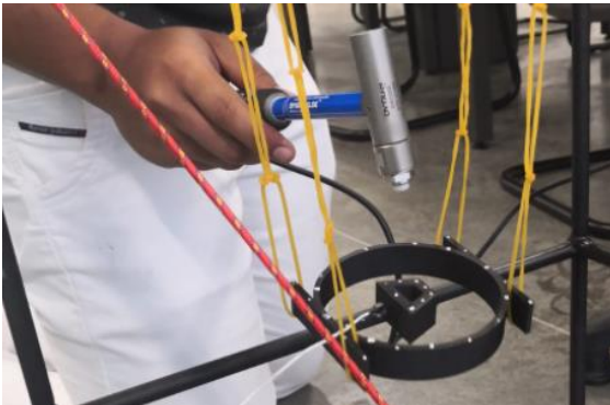
Figure 8. Mounting of the resonator modal analysis. Source: self-made.
