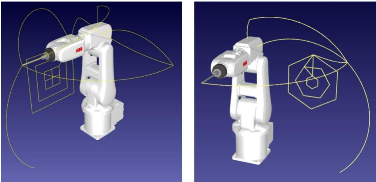
Figure 2. Trajectories to be used in the kinematic calibration process (XZ plane and YZ plane). Source: Own elaboration.
