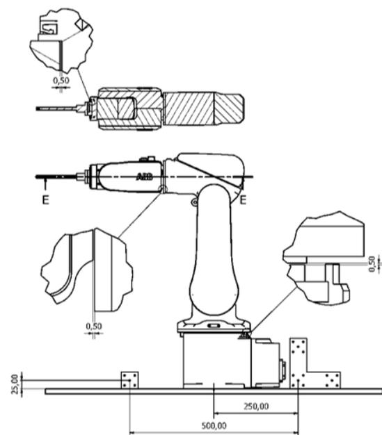
Figure 9. CAD model misalignment. Source: Own elaboration.
