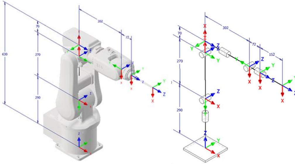
Figure 1. ABB IRB 120 robot reference system. Source: Own elaboration.
