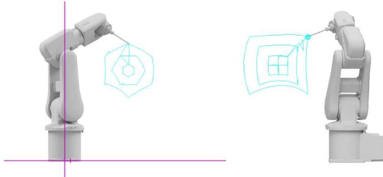
Figure 8. Automatically obtained points on the XZ plane trajectory. Source: Own elaboration.
