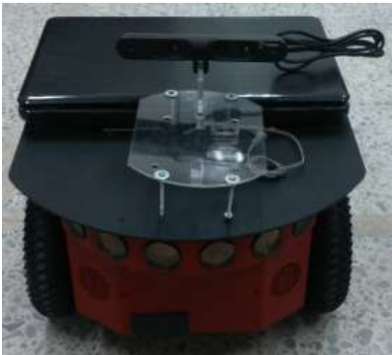
Figure 3. Pioneer 3DX + Carmine 1.08 Sensor
