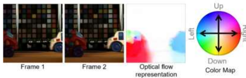
Figure 3. Illustration of the optical flow estimation between two frames following a color map. The scene changes from the Frame 1 to the Frame 2 and the optical flow representation adopts the respective color of the movement from the color map.
