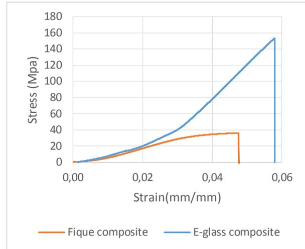
**Figure 5.** Figue and E-glass composites stress-strain curve. **Source.** Own.
