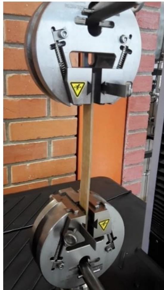
Figure 3. Fique composite tensile test. Source. Own.
