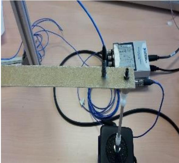
**Figure 4.** E-glass composite Dynamic vibratory test. **Source.** Own.
