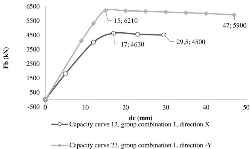
**Figure 7.** 3Muri capacity curve
