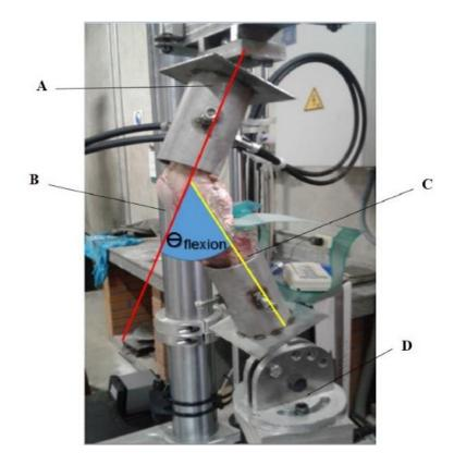
Figure 1. Experimental setup. (A) Ball bearing, (B) Knee joint, (C) K-4000 Tekscan sensor, (D) Tibia holding device with adjustable flexion angle.
