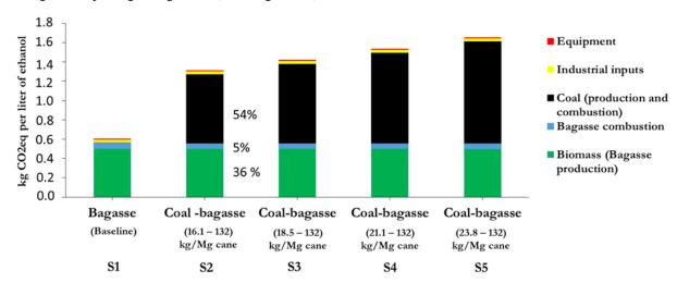
Figure 3. Comparison of the GHG emissions of different coal-bagasse mixture co-firing in the CHP system and the burning process of 100% bagasse.
