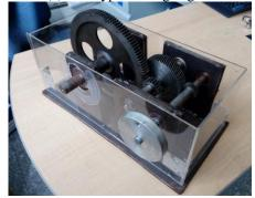
(b) Gear speed reducer
