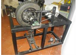
Figure 6. Model of a quarter of vehicle. Source: own elaboration.
