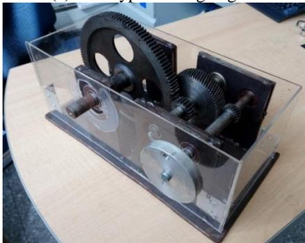
(b) Gear speed reducer
