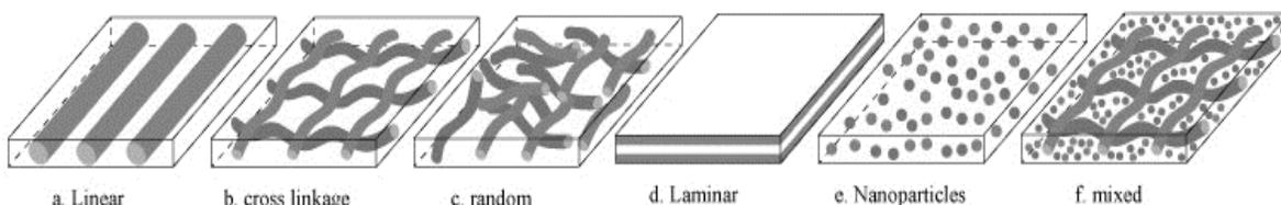
Figure 6. Composite classification according to fibers alignment. Font: Prepared by the authors and adapted from [2].
