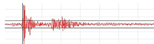
Figure 4. Waveform of a real AE signal.
