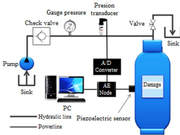
Figure 2. Schematic drawing of vessel.
